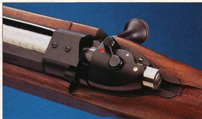
The very functional Winchester-style three-position safety and a new distinctive cocking shroud dress up the new Express action.
