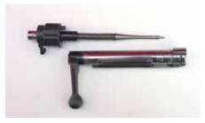
The firing pin is screwed into the front of the cocking piece which results in a stiff one-piece performance without the slop and play in a standard Mauser action. It is easy to remove the bolt from the bolt body for cleaning, which can be a must on the Alaskan coast or in the African rains.
