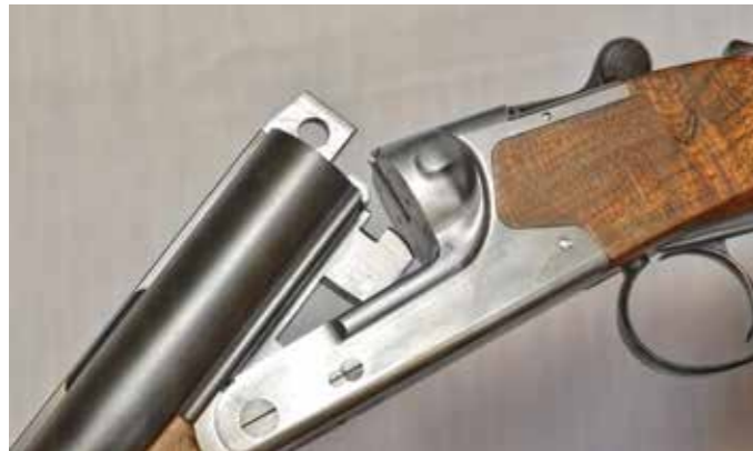
The 88B action is an Anson & Deeley boxlock with a triple lock – a double underbite with a Greener cross-bolt.
