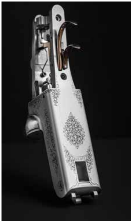
Above and right: Examples of actions that Heym builds. The actions come in five different sizes, depending on the calibre.
