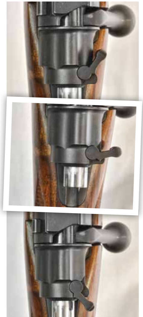
The three-position safety. From the top: Safety off and bolt unlocked; safety on and bolt unlocked; and lastly safety on and bolt locked.
