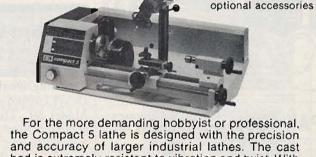
For the more demanding hobbyist or professional, the Compact 5 lathe is designed with the precision and accuracy of larger industrial lathes. The cast bed is extremely resistant to vibration and twist. With optional accessories the Compact 5 also converts to a universal machine tool with the added capabilities of thread cutting, milling, drilling, gear cutting, and vertical boring. The basic lathe is \$795.00.
